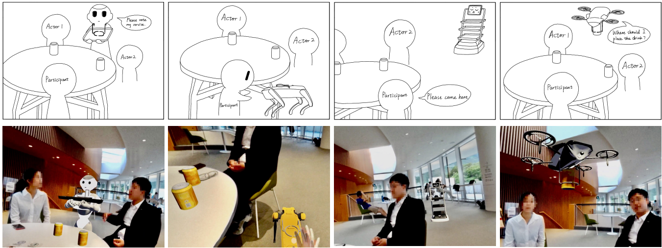
(a) Pepper, the anthropomorphic robot, was asking the participant to provide feedback. (b) The participant was asking Spot, the zoomorphic robot, to go away. (c) The participant was asking the grounded technical robot to come over. (d) The aerial technical robot carried the second cup of drink to the participant and asked him/her where to place it.
